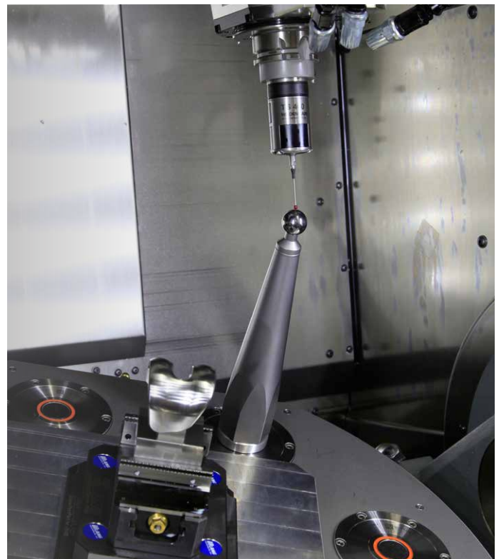
The KinematicsOpt TNC function measures rotary and swivel axes simply and quickly with the help of a calibration sphere. The kinematics table compensates for possible deviations, and with a protocol if specified by the customer.
