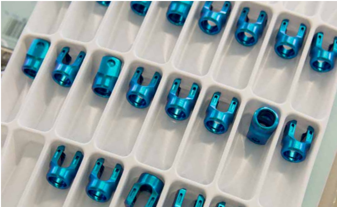
Titanium implants for spinal column applications. Leitner AG achieves perfect surfaces with the iTNC 530 and saves on complex reworking.
