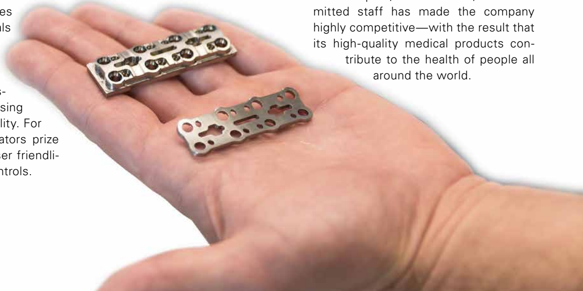
The uNion plate system for cervical vertebrae after initial clamping (above) and following final machining (below).
