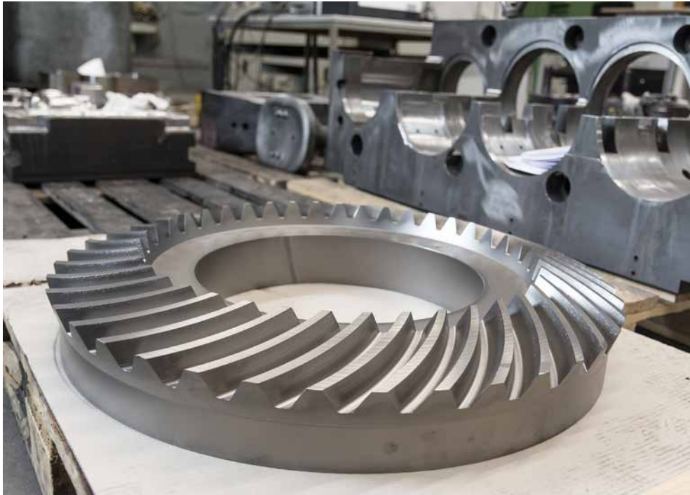
Five-axis machining enables almost any gear geometry.
