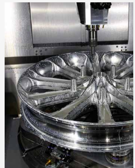
The 3-D milled Unbreakable wheel is machined from a solid aluminum mono-block.
