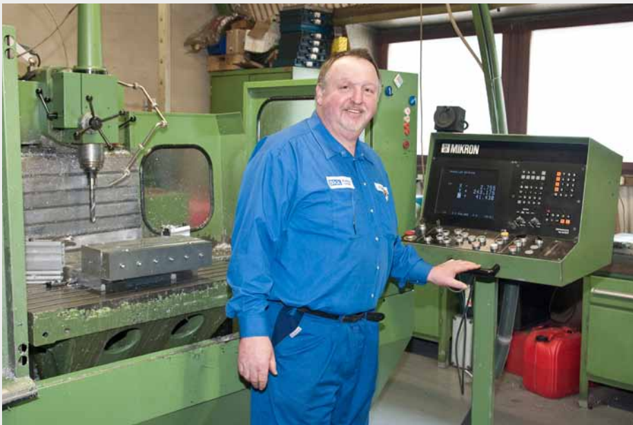
Karl Kubina at his "old Mikron" with a HEIDENHAIN TNC 155 control—still in operation after 31 years.
