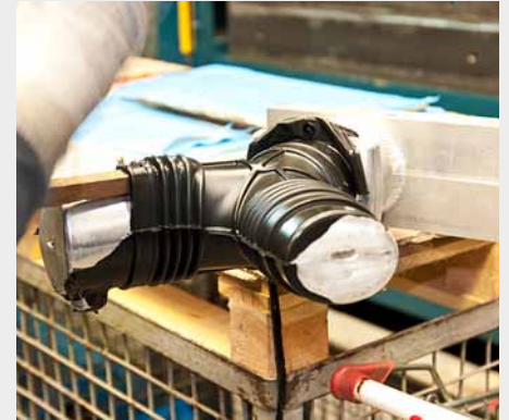
The finished cast rubber part right when it is being removed from the mold.
