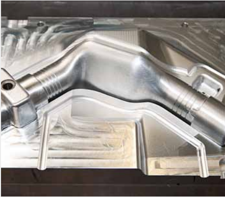
Cast forms with complex contours—the TNC 620 machines them easily.
