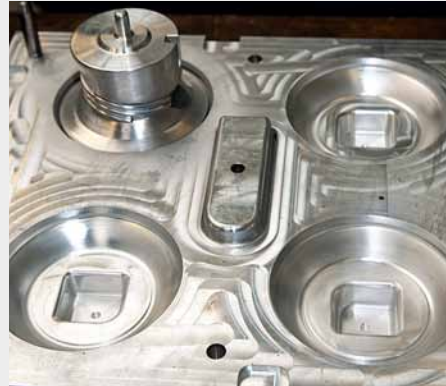
Cast forms with complex contours—the TNC 620 machines them easily.
