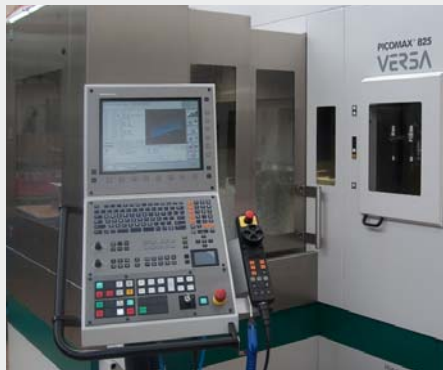
An efficient team — a Fehlmann machining center with a HEIDENHAIN iTNC 530.
