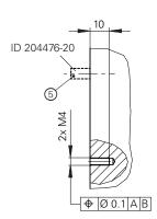
$\ensuremath{\mathbb{M}}$  = Measuring point for operating temperature/vibration
