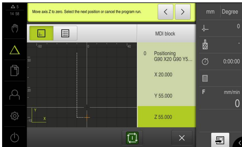
Figure 57: Example – Execution of an MDI block with scaling factor
