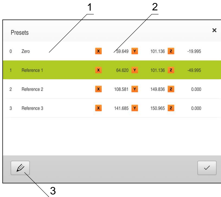
Figure 28: Preset table with absolute positions in the Milling application mode
