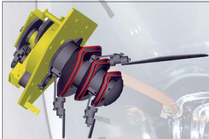
3-D control cam with tilting and rotating technique
